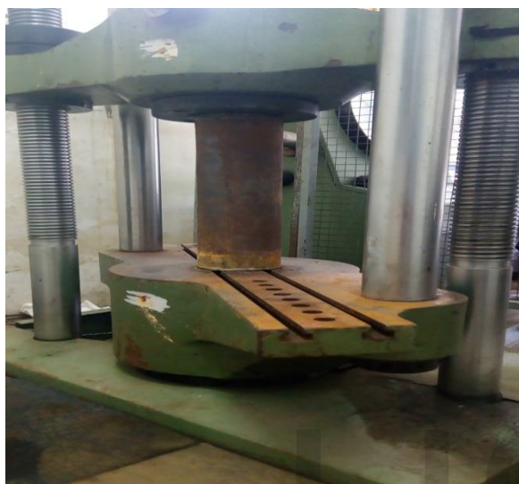
Fig 9. Test setup for CFT columns
